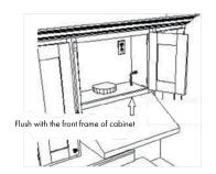
Lift the hood up and place it below the cabinet. Make sure to center the hood beneath the cabinet. Make sure that it is flush with the front of the cabinet.
