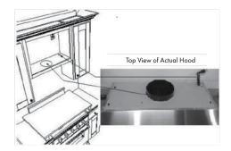
Create an opening for the electrical wire and hood exhaust under the cabinet.
